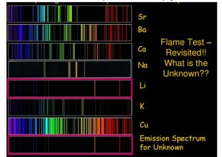
Used to analyse and identify metal ions in solution
